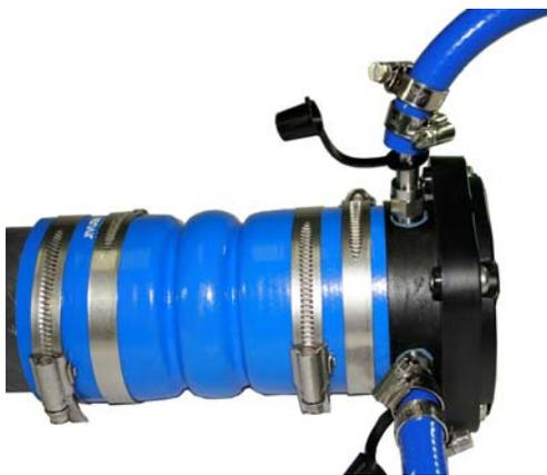
Remove the water pick-up hose and plastic cap from the water injection fitting that brings water from the engine's raw water cooling system to the SureSeal™.
