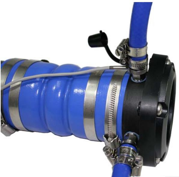
Press the plastic cap and the water pick-up hose back onto the injection fitting until it abuts the sensor ring, holding the ring in place. Tighten both hose clamps over the hose on the injection fitting.
