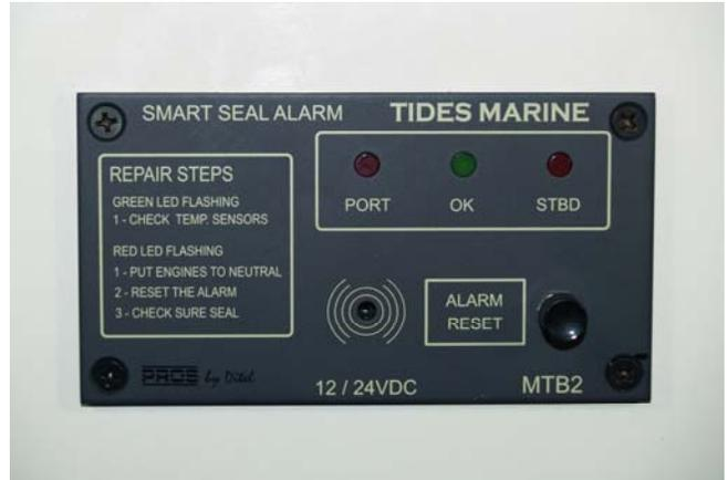
Insert the control panel into the finished hole and secure it with the 4 screws provided.
