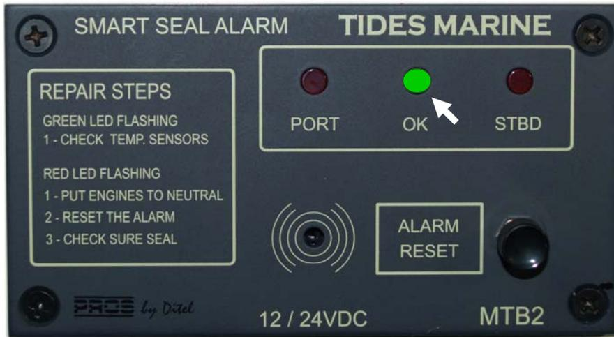
Turn the power on to the Smart Seal main panel.
