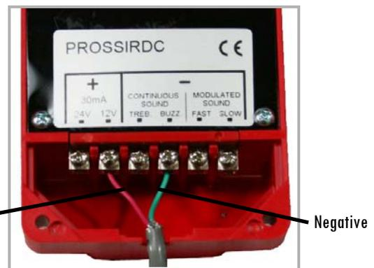
Strip the wires on the opposite end to connect them to the back of the siren. There are four (4) sound settings as shown by the label on the back of the siren.
