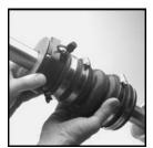
Carefully slide the assembly (hose end first) onto the shaft and onto the stern tube.
