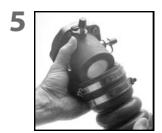
Place two hose clamps over each end of the articulating hose. Insert the SureSeal $^{TM}$  into the hose as far as it will go. Tighten hose clamps around the SureSeal $^{TM}$ .
