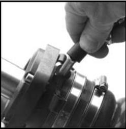
Connect the SureSeal™ to a pressurized water supply source (a point in the engine’s raw water cooling system) by attaching the water injection hose to the stainless fitting on the SureSeal™ housing. If there is a second injection hose fitting on the SureSeal™, it is used to complete a crossover feed between the port and starboard SureSeals™.
