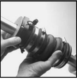
Carefully slide the assembly (hose end first) onto the shaft and onto the stern tube.
