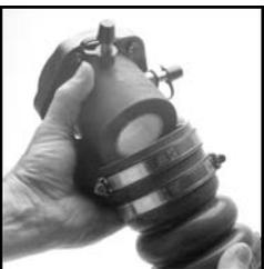
Place two hose clamps over each end of the articulating hose. Insert the SureSeal™ into the hose as far as it will go. Tighten hose clamps around the SureSeal™.
