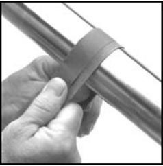
Examine area carefully. Be sure it is free of pitting, nicks or surface imperfections which could cause leaking. Clean area thoroughly. Polish the shaft using 300 grit wet/dry sandpaper or emery cloth, working around the shaft. Fore and aft actions could put flats or grooves in the shaft. The assembly may be shifted forward on the shaft by adjusting the position of the hose on the stern tube at time of installation.
